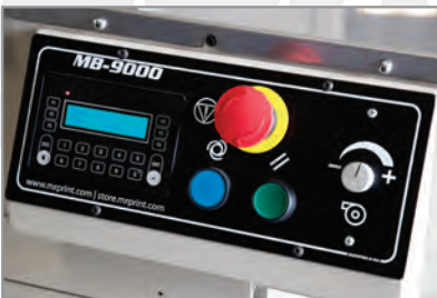
HMI controller provides digital control over critical settings
